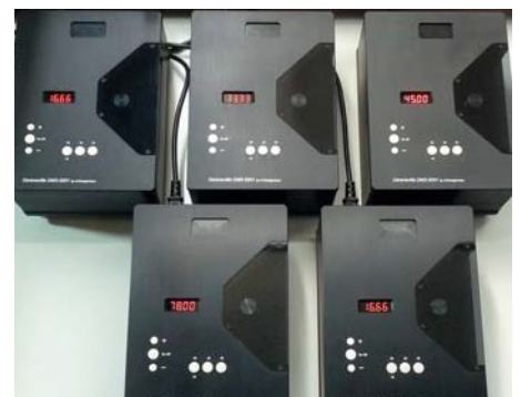
24 hours endurance test run of the first 5 Dereneville DMS-5001
