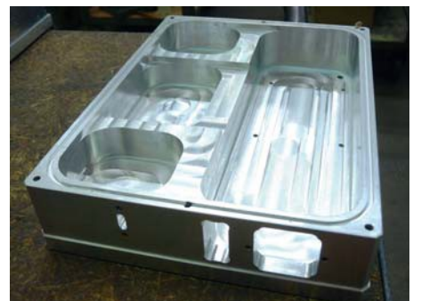
Finished lower part with lateral openings
